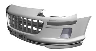
Here is an example of a bumper where the "grill" cannot be removed and requires extra difficult masking.
